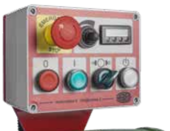
Inverter board: real speed is shown on display.
