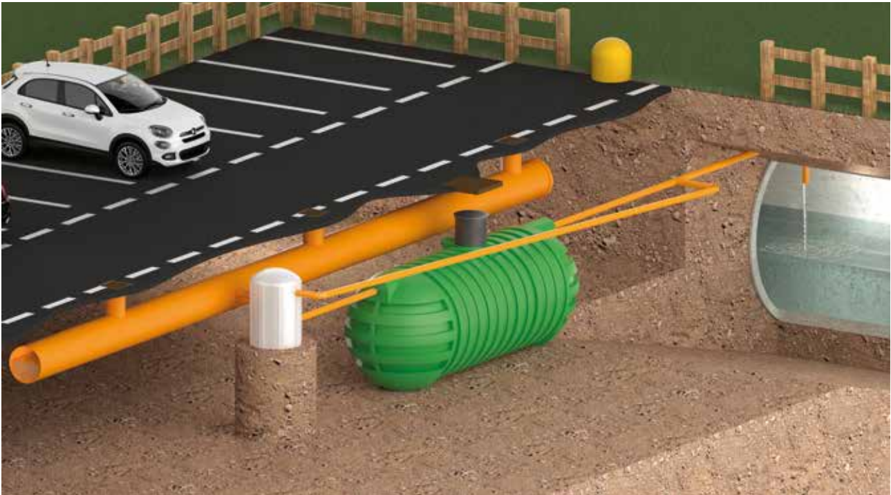
Rainfall and washout water processing system example
