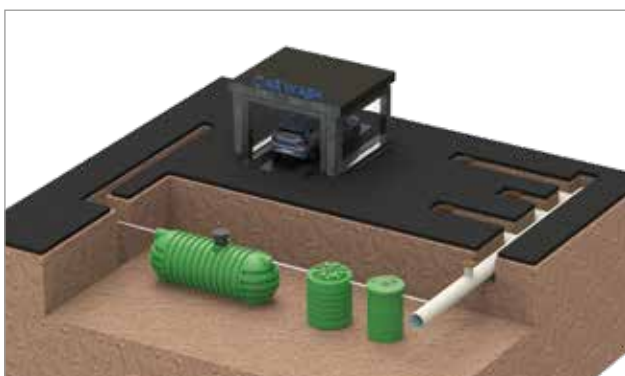
Example of a system with degreasers and oil separators
