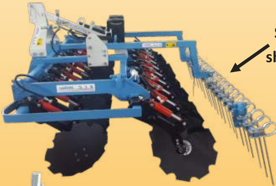
Toothed cage roller with shock-absorbed couplings
