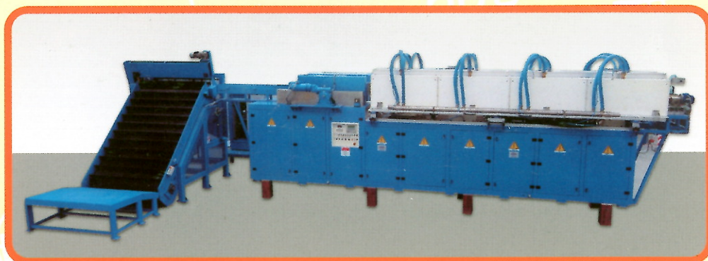
FC100 – 4000 kW – 1 kHz con ribaltacassoni, tavola vibrante e caricatore automatico multilame. FC100 – 4000 kW – 1 kHz with bin tipper, vibrating table and multiblade automatic loader
